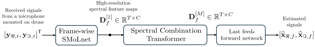
Fig. 2. Proposed direct-mapping approach with frame-wise SMoLnet and spectral combination transformer.
