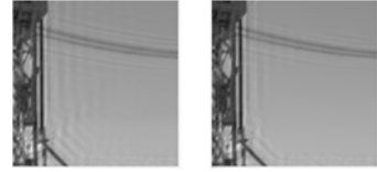
Fig. 6. Lleft) Original image patch; (Right) After ringing effect removal.
