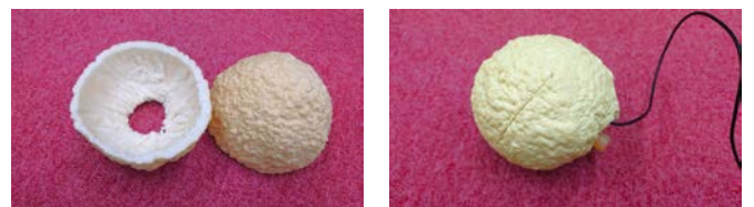
(a) Windshield components. (b) Attached to microphone array.
