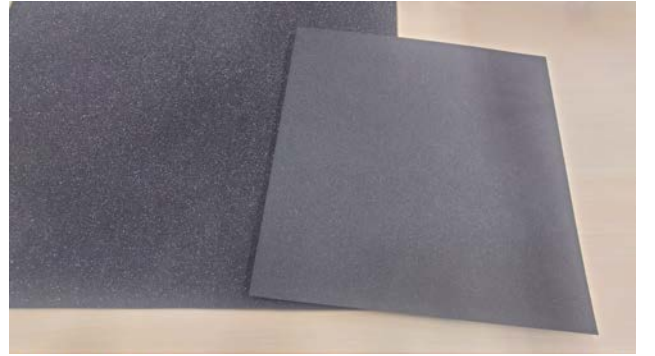
Fig. 9: PU foam (left in the figure) and PE foam (right in the figure)
