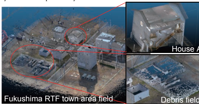
Fig. 4. Generated 3D Point Cloud for Fukushima RTF town area field
