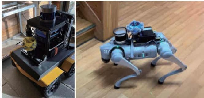
Fig. 3. Clearpath JACKAL(left) and Unitree Go2(right). Each has a 16 ch cylindrical microphone array and LiDAR.
