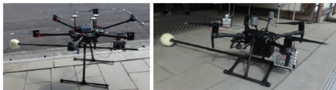
Fig. 2. DJI Matrice 600 Pro(left) and DJI Matrice 210 RTK V(right). Each has a 16 ch spherical microphone array (white) at the end of the pole which is covered by windshield made of special urethane with light weight.
